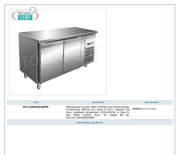
REFRIGERATED TABLE with 2 DOORS and NEUTRAL DRAWER , SNACK line, capacity 228 litres , temperature -2°C /+8°C, ECOLOGICAL in Class B :
